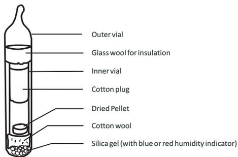
2. Wear protective glasses when opening ampoules! Heat the tip of the ampoule in a flame.
