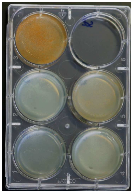
Sodium chloride tolerance test (from top left to bottom right: 0%, 5%, 2,5%, 10%, 7,5%)
