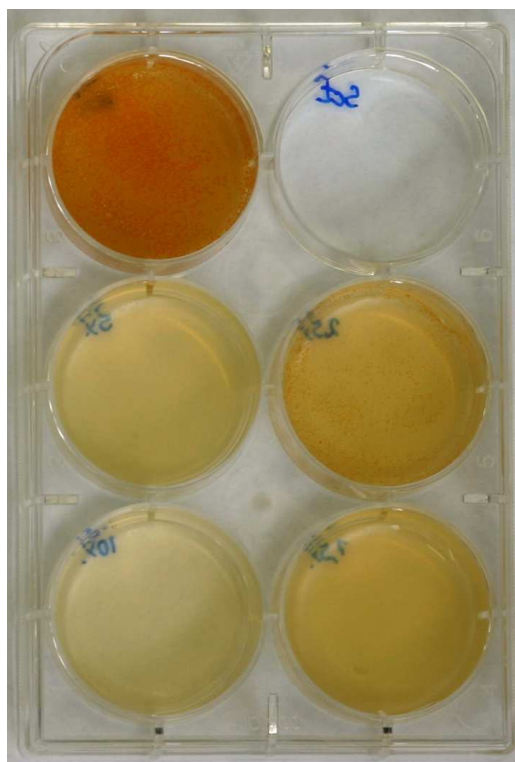
Sodium chloride tolerance test (from top left to bottom right: 0%, 5%, 2,5%, 10%, 7,5%)
